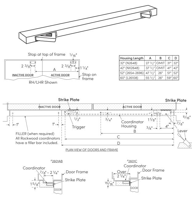
NOTE: Field adjustment of door closers is required after installation of coordinator to insure against doors closing too fast and changing coordinator mechanism. Field adjustment of coordinator override could be needed.
