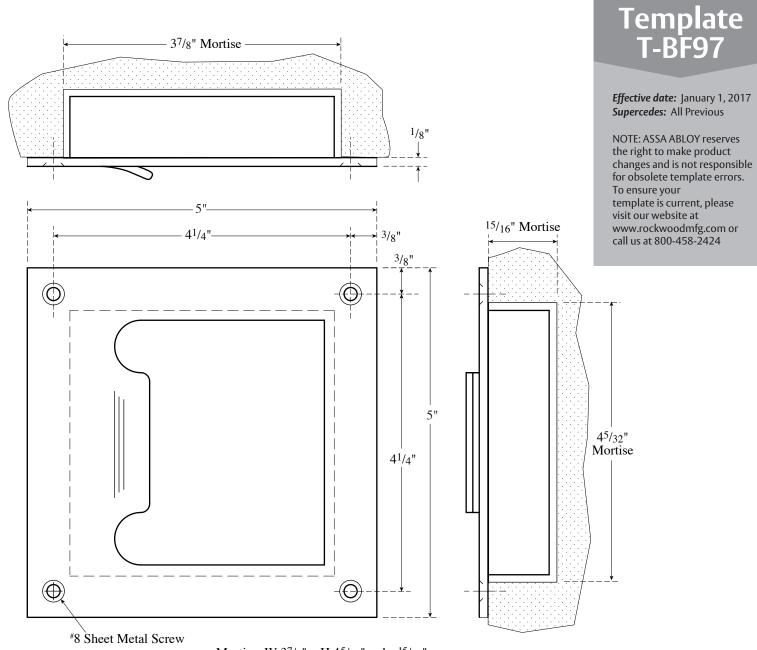
Mortise: W 37/8" x H 45/32" x dp. 15/16" Drop pull into opening and drill mounting holes using holes in handle as a template.
