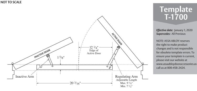
Spot (four) Holes in Door Stop for #10-24 Machine Screws or #10 Wood Screws
